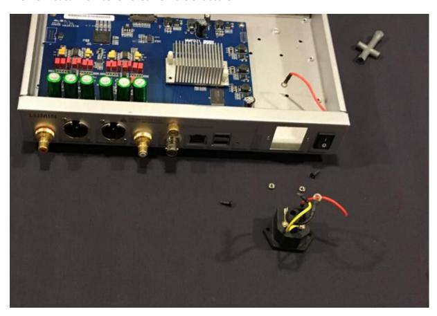
Installation of the Sbooster DC input bracket (product looks different from the sample in this manual)
